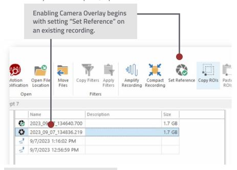
Show overlay reference image with live feed for proper camera alignment.
