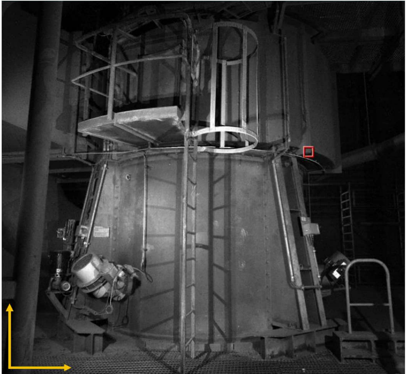
X Figure 1. Measurement point of separator and cone structure.
