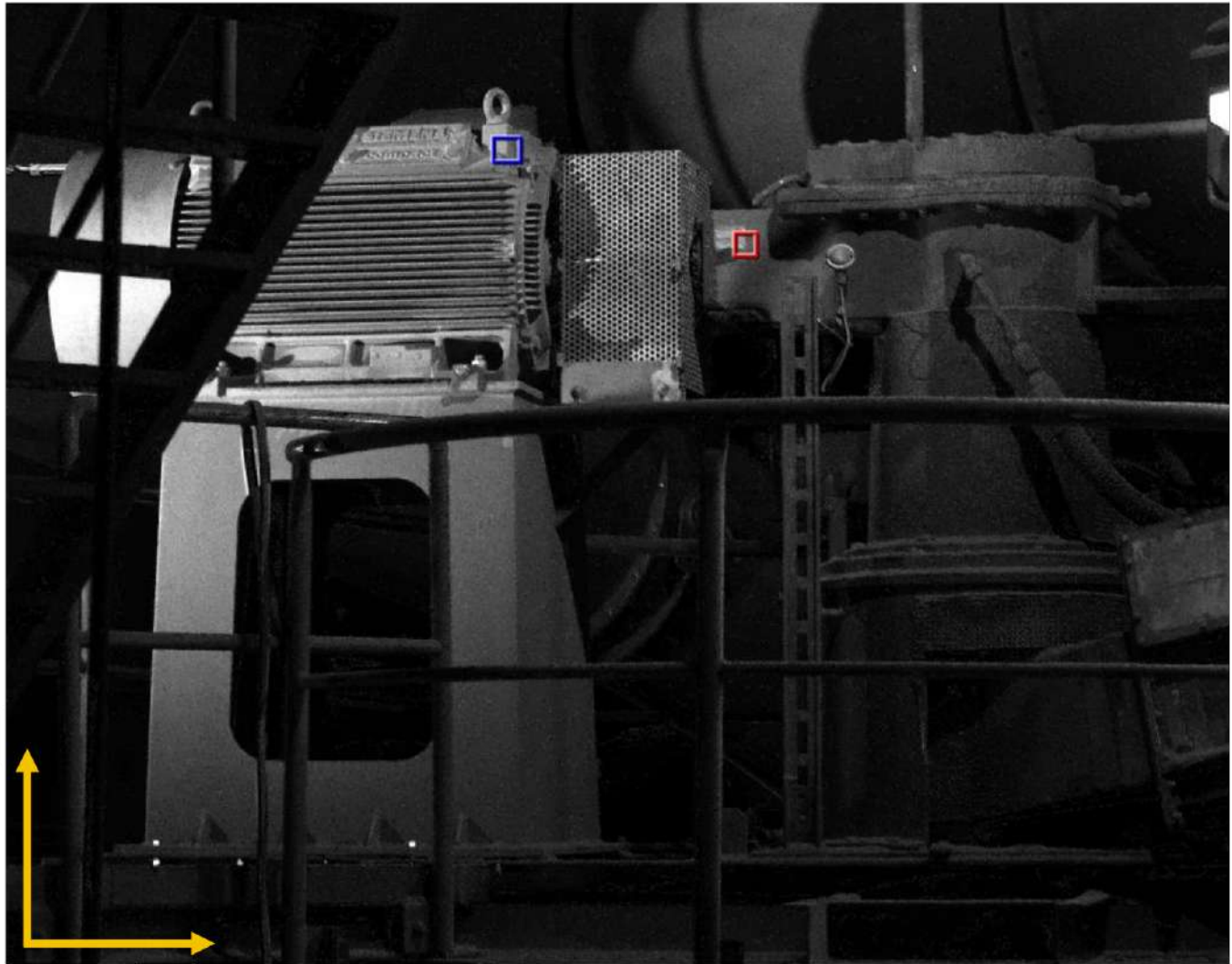
Figure 3. Measurement points of motor and angular gearbox unit.
